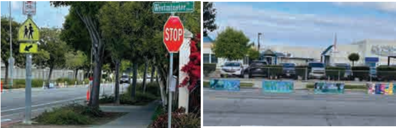
Figure 1. Temporary Bike Lane Separations on McKinnon Street
